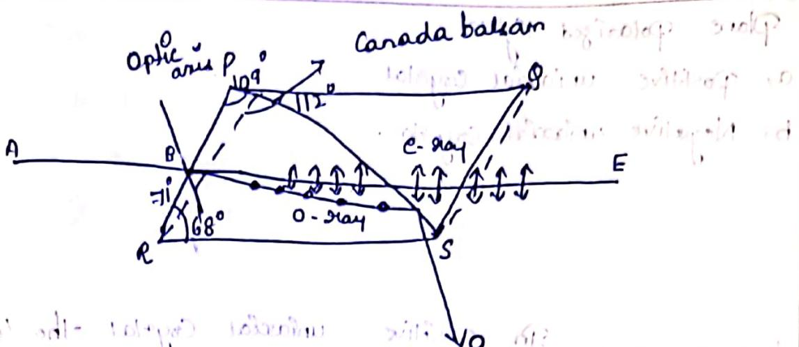
1. When a beam of light AB enters the face PR of the Nicol prism, it is doubly refracted into ordinary ray BO and extra ordinary ray BE.
